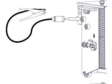
Connect the cable assembly to the welding power source and the wire feeder and the gas supply.
