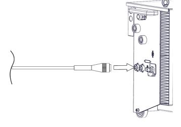
Connect the Ethernet cable to the power source and the robot controller.
