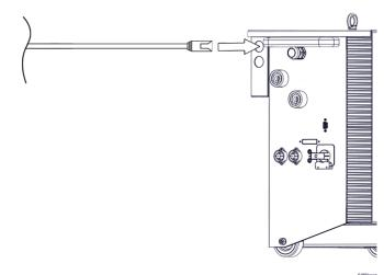
Connect the welding power source to the power supply.
