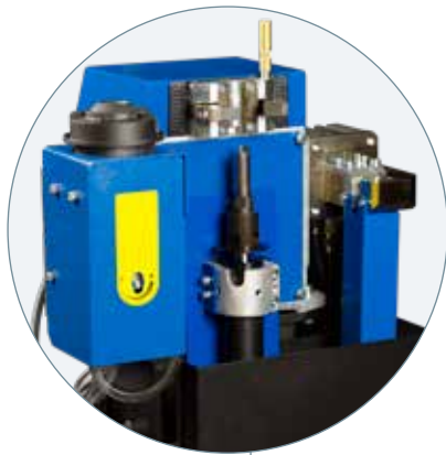
TCS-FP – uncovered to show reamer blade and mechanism
