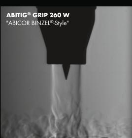
The illustrations (left) show the much more laminar gas flow with the ABITIG® GRIP 260 W torch for top gas cover and avoidance of pores compared with the "LINDE® -Style" torch ABITIG® GRIP 20.
