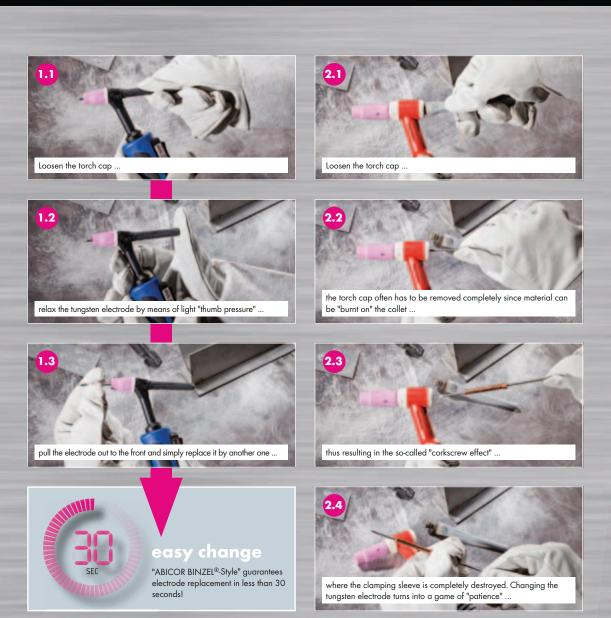
When the electrode does need to be replaced, this can be done in just a few steps in no time. Simple loosen the torch cap and relax the electrode by exerting slight "thumb pressure" on the end of the torch cap – the electrode can then be removed and replaced effortlessly. Simple and fast – without tools! (Fig.: 1.1–1.3)
